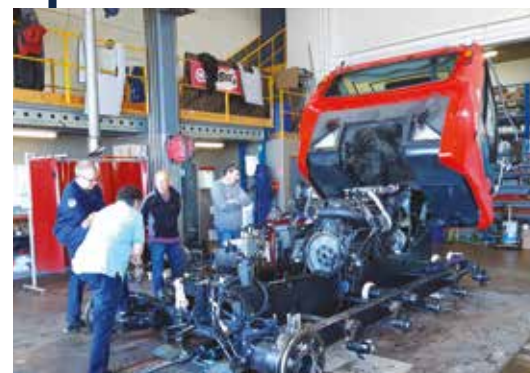
Retrofitting one of the Group's snow groomers, a Kassböhler PB600
